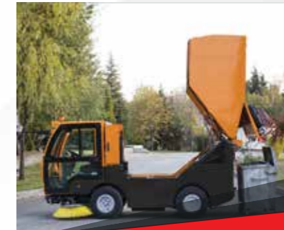
Capability of dumping into garbage container
